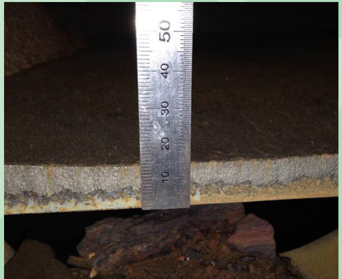
Competing plate after 2 weeks – 4mm of wear
