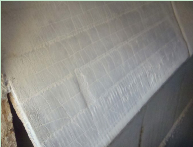
SPOT60® overlay wear liners after 3500 hours and 8.3 Million tonnes
