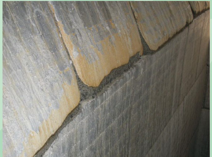
Standard overlay plates after 1300 hours
